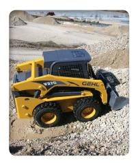
extra Long wheelbase of more than 49 inches enhances machine stability when lifting and loading and provides a smoother ride over rough terrain.
