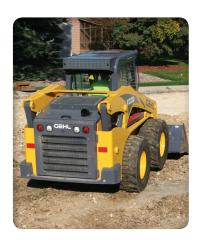
HEAVY-DUTY CHASSIS on the model V330 provides excellent weight distribution, enhancing stability. A rear bumper adds protection and towing capability.
