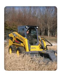
AUXILIARY HYDRAULICS have the power to run a variety of attachments. Standard auxiliary control allows an operator to adjust the flow rate for optimal performance or detent for continous use.
