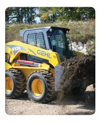
**SHIFT INTO HIGH GEAR** with standard two speed drive, providing speeds over 12 mph. The drive motors feature "soft-shift," providing a smooth transition between speed ranges.
