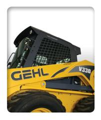
EXCELLENT VISIBILITY to the sides, rear and front is achieved with a unique, low-profile boom design. A roof window allows the operator to view the lift arm when fully raised.
